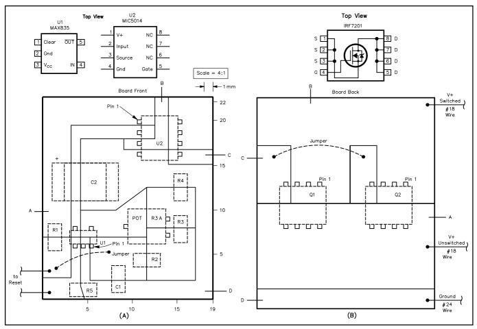
Figure 13—Part placement for the PC-board top (A) and back sides (B), respectively.
